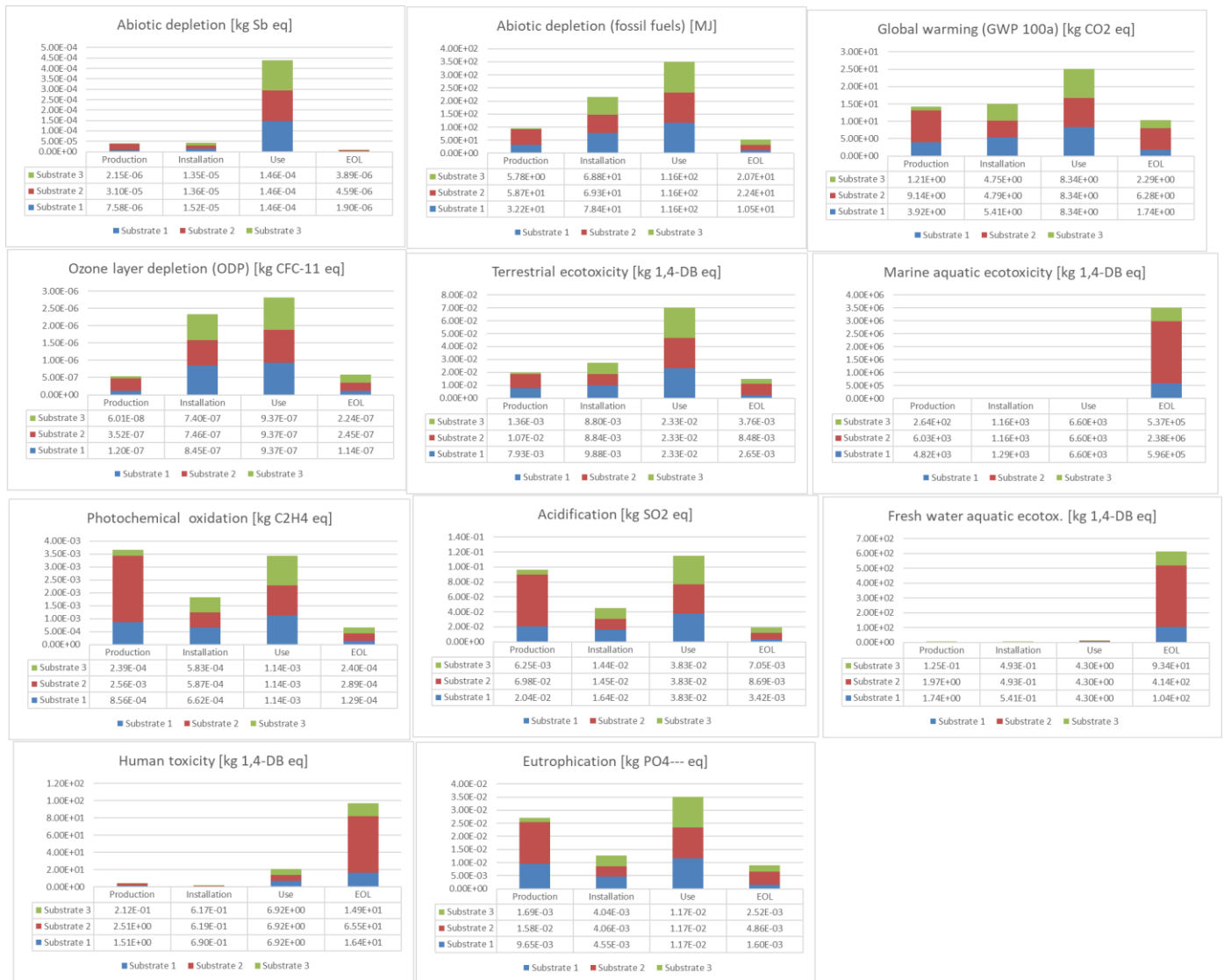
Figure D. 1. Environmental impact distribution of the three substrates across different life cycle stages for each impact category.
